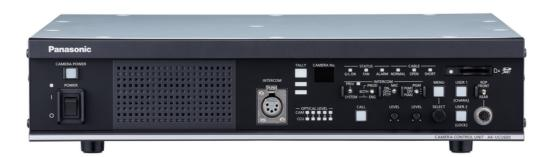
The CCU supports UHD and HD simultaneous output while still having a compact size. HD mode enables output in 240p, 180p and 120p during normal filming.
