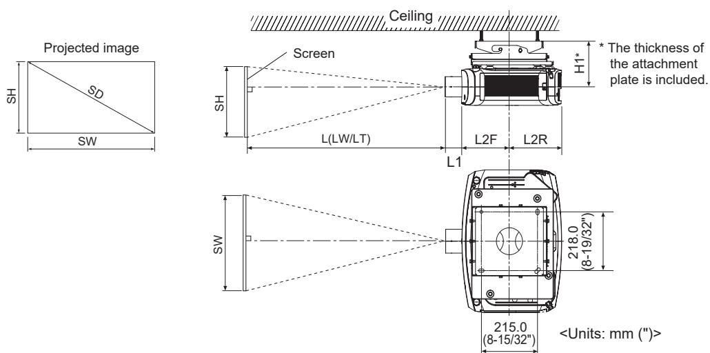
(when using the ceiling mount bracket ET-PKD120H (for high ceilings))
