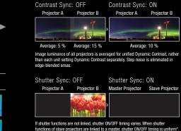
\* Includes fade-in and fade-out effects. Projector shutter functions can be set to operate individually if desired
