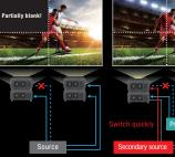
If the main input signal is disrupted. image display is cut off
