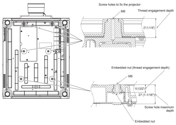
Screw tightening torque: (M6) 4 ± 0.5 N·m
