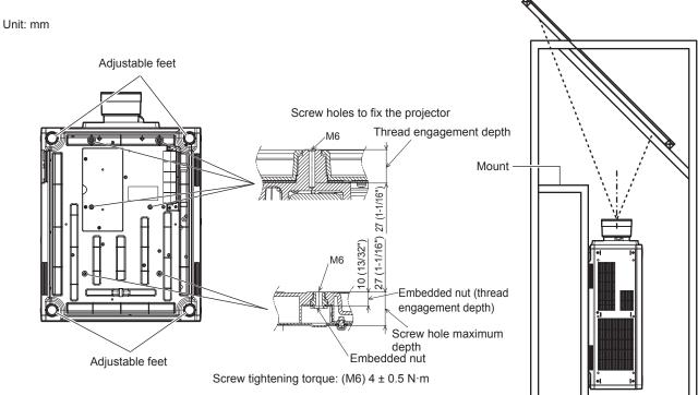
Positions of screw holes to fix projector and adjustable feet
