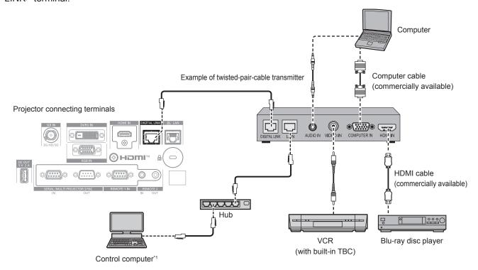
1 Control target is the projector or the twisted-pair-cable transmitter. The control itself may not be possible depending on the twisted-pair-cable transmitter. Check the operating instructions of the device to be connected.
