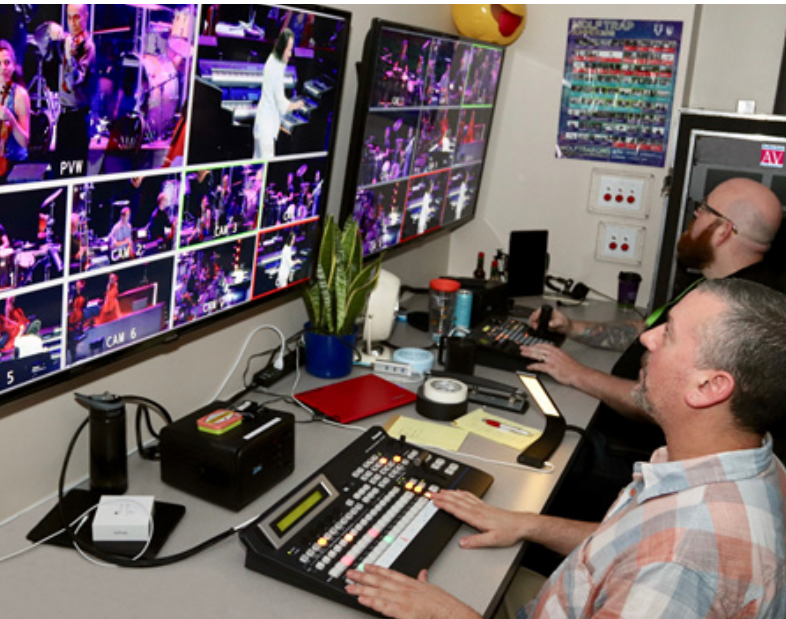
The AV-HS450 switcher is located in a new camera control center under the stage.
