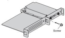
• Tightening torque guideline: 0.5 N·m or less
