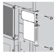
• Tightening torque guideline: 0.5 N·m or less
